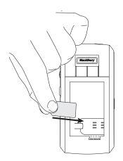
5. Slide the SIM card into the holder so that it lies flat below the metal guide.
