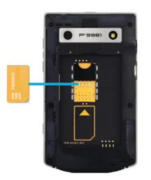
Slide the SIM card into the slot.
