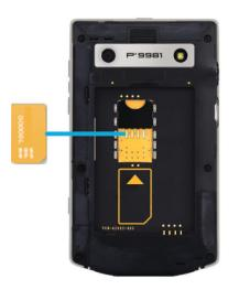
Slide the SIM card into the slot.
