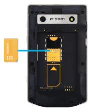
Slide the SIM card into the slot.
