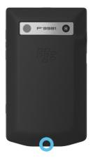
To remove the battery door, pull up the bottom of the battery door.
