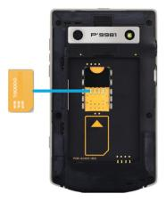
Slide the SIM card into the slot.
