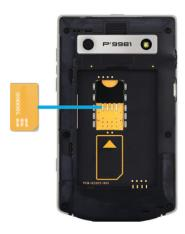
Slide the SIM card into the slot.
