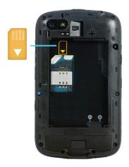
Slide the SIM card into the slot.
