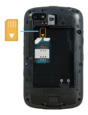
Slide the SIM card into the slot.
