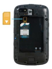
Slide the SIM card into the slot.
