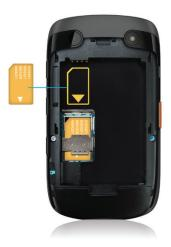
Slide the SIM card into the slot.
