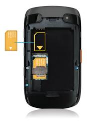
Slide the SIM card into the slot.
