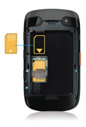
Slide the SIM card into the slot.
